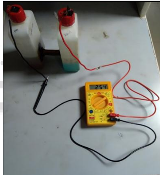
Fig. 5.19: MFC with voltmeter showing voltage and current
