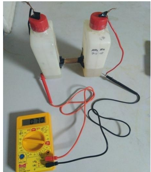
Fig. 4: Dual Chambered MFC with Voltmeter
